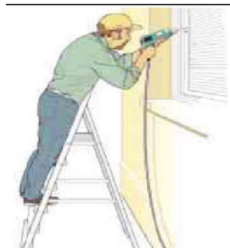
Correct – steps facing work activity
