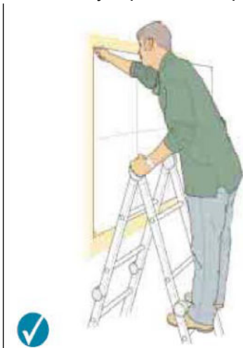
Correct – two clear rungs. Don't work any higher up this type of stepladder.
