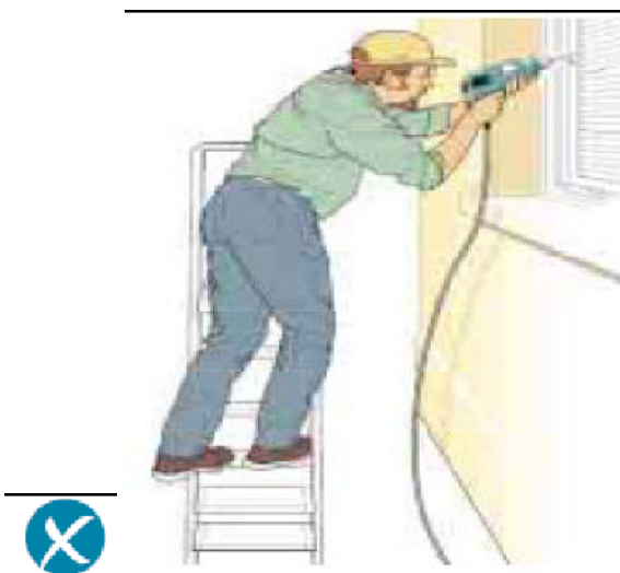
Incorrect – steps side on to work activity
