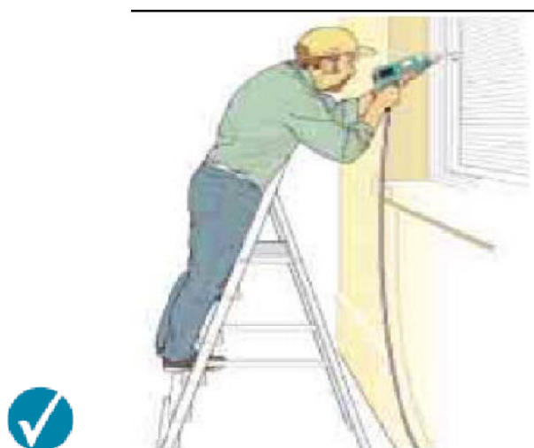
Correct – steps facing work activity
